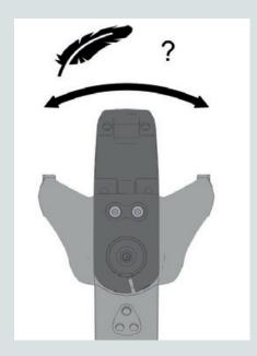
If the stem can be easily rotated after tightening, you can proceed with the next step.
