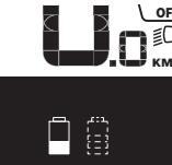
If an eBike has two battery packs inserted into it and both battery packs are charged on the bike, the charging progress of both battery packs will be indicated on the display (the left-hand battery pack is being charged in the illustration). You can tell by the flashing indicator on the battery pack which of the two battery packs is being charged.
