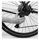
If you have **derailleur gears**, you should shift the chain to the medium or small chainring or to the smallest sprocket before removing the wheel. This shifts the rear derailleur right to the outside where it does not interfere with the removal of the wheel and the chain tension is not too high.
