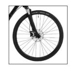
The wheel consists of hub, spokes and rim. The tyre is mounted onto the rim so that it encases the inner tube. There is a rim tape running around the base of the rim to protect the sensitive inner tube against the spoke nipples and the edges of the rim base, which are often sharp.
