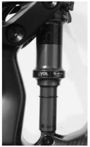
Go for a test ride every time you made a change. Ride your bicycle on different kinds of surface and check the travel of the rubber ring/cable tie afterwards. The distance to the wiper is the maximum rear shock stroke you have used. If the rubber ring/cable tie has moved a few millimetres only, the setting of your rear shock is too hard. Reduce the air pressure or in the case of rear shocks with steel coil the spring preload. If this does not help, have the spring replaced.
