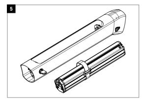
The battery is now completely separated from the frame and can be transported for charging, for example.
