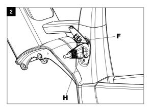
The charging socket is thus accessible for the charging plug (H). Insert the charging plug (H) by applying light pressure. The ribbed side of the plug must point towards the front wheel and the side with the recess towards the rear wheel. Please refer to the "Bosch eBike Battery Guide" manual for information on how to charge the battery.
