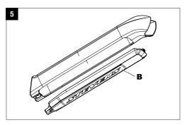
Hook into the opening (A5) with one finger and then pull the opening forwards and downwards with your finger to release the cover (B) from the fixation. The cover will release with a jerk.
