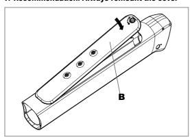
If you have removed the battery for charging, we recommend always remounting the cover (B).
