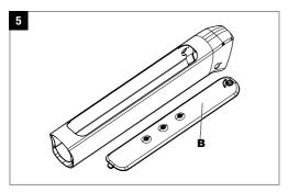
Turn the shutter (A4) counterclockwise. This releases the cover (B) from the fixation.
