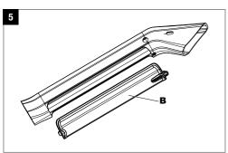
Turn the shutter (A3) clockwise or counterclockwise. The cover (B) will be automatically released from the frame.
