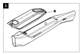
Turn the shutter (A3) clockwise or counterclockwise. The cover (B) will automatically release from the fixation.
