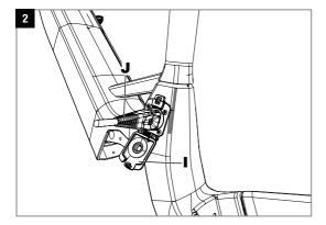
The charging socket is now accessible for the charging plug (J). Insert the charging plug (J) by applying light pressure. The grooved side of the plug must point in the direction of the front wheel and the side with the indentation towards the towards the rear wheel. For details on how to charge the battery, please refer to the Bosch manual "Bosch eBike Battery Guide".
