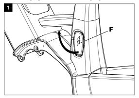
Slightly lift the cover (F) on the left side of the seat tube above the motor interface from below and carefully fold it upwards.
