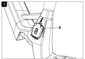
Remove the cover (I) on the left side of the seat tube above the motor interface by pressing the locking mechanism and open it downwards.
