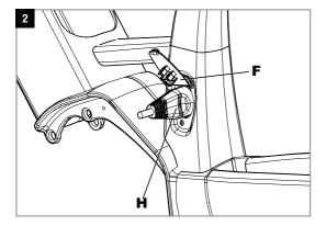
The charging socket is thus accessible for the charging plug (H). Insert the charging plug (H) by applying light pressure. The ribbed side of the plug must point towards the front wheel and the side with the recess towards the rear wheel. For details on how to charge the battery, please refer to the Bosch manual "Bosch eBike Battery Guide".
