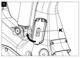
To open the cover (K) on the left side of the seat tube above the motor interface, apply light pressure to unlock it. Then lift it up slightly and carefully open it upwards.
