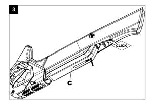
To completely lock the battery (C), apply pressure (upwards) to the battery pack in the area of the red retaining catch with lock. A "CLICK" sound is heard when the battery is securely locked into position.
