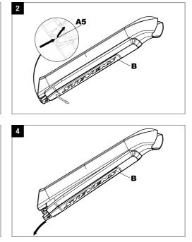
Hook into the opening (A5) with one finger and then pull the opening forwards and downwards with your finger to release the cover (B) from the fixation. The cover will release with a jerk. 2
