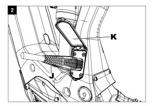
The charging socket can now be accessed with the charging plug (J). Insert the charging plug (J) by applying light pressure. The grooved side of the plug must point towards the the rear wheel and the side with the indentation must point towards the front wheel. For details on how to charge the battery, please refer to the Bosch manual "Bosch eBike Battery Guide" or the STEVENS manual.
