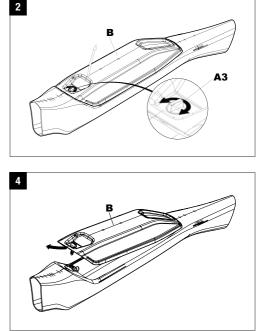
Turn the shutter (A3) clockwise or counterclockwise. The cover (B) will automatically release from the fixation. **2**
