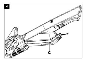
In the next step pull the battery (C) forward and out of the holder.
