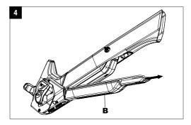
Press the button (A6) to release the cover (B) from the fixation. 2
