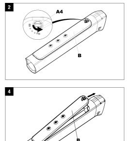
Turn the shutter (A4) counterclockwise. This releases the cover (B) from the fixation. 2
