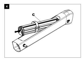
When removing, make sure that the battery (C) does not touch the seat tube, top tube or frame opening.
