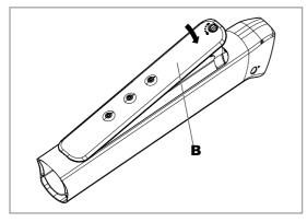
If you have removed the battery for charging, we recommend always remounting the cover (B).
