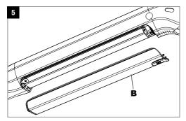
Slide the latch (A7) down to release the lid (B) from its fixation. 2
