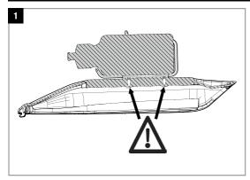
The threads for the bottle holder or accessories are limited in how deep they can go. A bolt can only be screwed in to a certain depth. The threads in the cap are M5 threads. If the screw is screwed in too far or tightened too much (MAX, 5 Nm), the cap, the thread or even the battery may be damaged. Please contact your STEVENS dealer to select the correct bolts.
